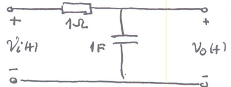
$|V_o(j\omega)|^2 = \frac{100}{(1+\omega^2)(25+\omega^2)} = \frac{100}{24} \left[ \frac{1}{1+\omega^2} - \frac{1}{25+\omega^2} \right] = \frac{25}{6} \left[ \frac{1}{1+\omega^2} - \frac{1}{25+\omega^2} \right]$
